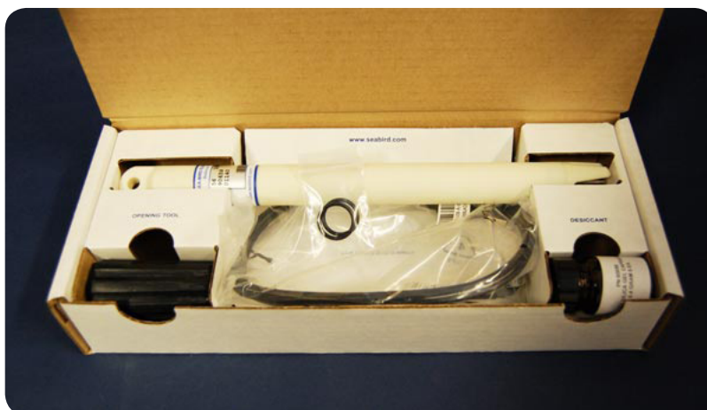
SBE 56, opening tool, desiccant, cable, and spare O-rings
