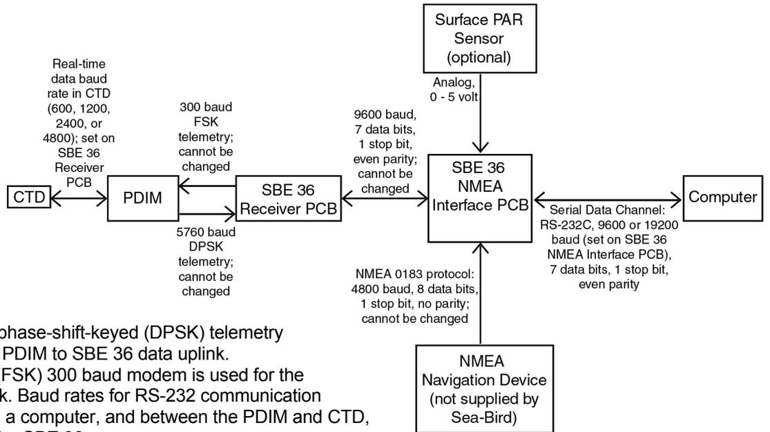
A 5760 baud differential-phase-shift-keyed (DPSK) telemetry technique is used for the PDIM to SBE 36 data uplink. A frequency-shift-keyed (FSK) 300 baud modem is used for the SBE 36 to PDIM downlink. Baud rates for RS-232 communication between the SBE 36 and a computer, and between the PDIM and CTD, are switch-selectable in the SBE 36.
