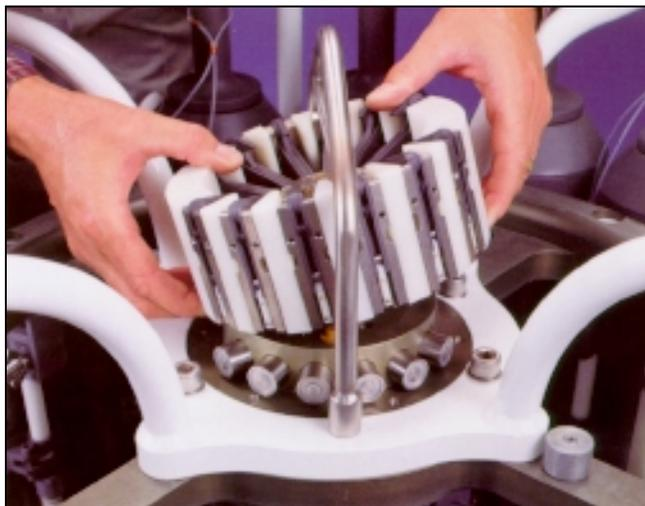
When used with a 911plus, the CTD system provides Carousel power and control.
